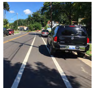
Kalamazoo Avenue contains on-street parking placed between a bike lane and the curb.
